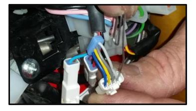
Locate the four-pin connector at the meter (behind the headlight mask) as shown and lift the small rubber boot away. Then, with a small safety pin or paper clip, remove the light gray wire from the connector.
