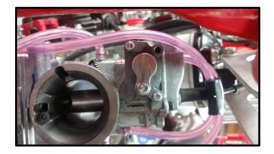
Reinstall the TPS plate (now without the lever) and the TPS plug that is included with this kit making sure the oring is in place.
