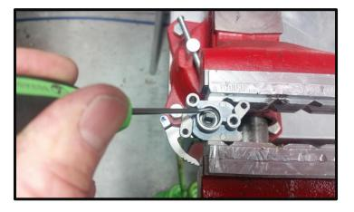
With the TPS lever and housing out, clamp the plate in a vice and remove the snap ring holding the TPS lever in place
