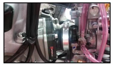
Remove the stock intake manifold and replace it with the new one supplied using the new gaskets. Re-install the slide into the carburetor and install the carburetor on the manifold. Install the subframe, rear air boot, and exhaust muffler.
