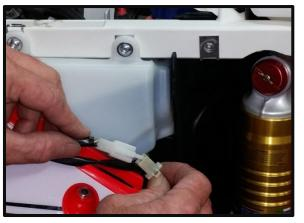
Start by removing the muffler, airbox bolts (the ones attached to the plastic part of the subframe) and the four rear subframe bolts holding the plastic part to the two aluminum uprights. Swing the plastic part of the sub frame up leaving the airbox in place. Remove the oil tank assembly including the oil pump and the low oil sensor (attached) along with the oil line going to the intake manifold
