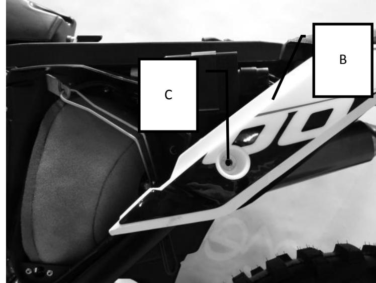
The Oil Pump Control Unit (39) can be found under the left plastic of the mudguard. To reach it, proceed as follows:
