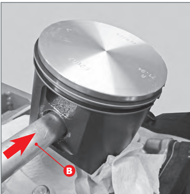
Removal of pin bolt.
