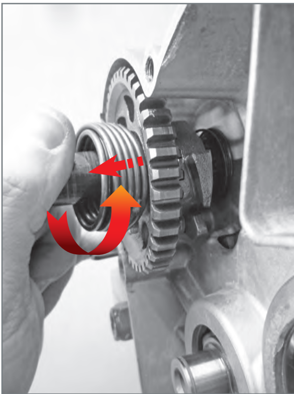
Extraction of shaft from crankcase.
