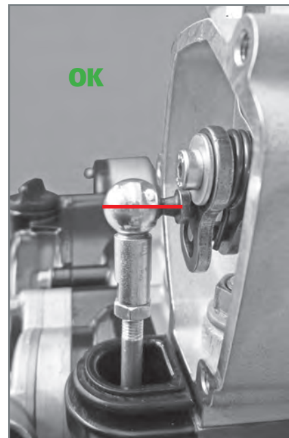
Correct position of the control rod seat.
